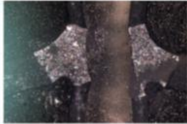
Cross section of a laser weld seam
